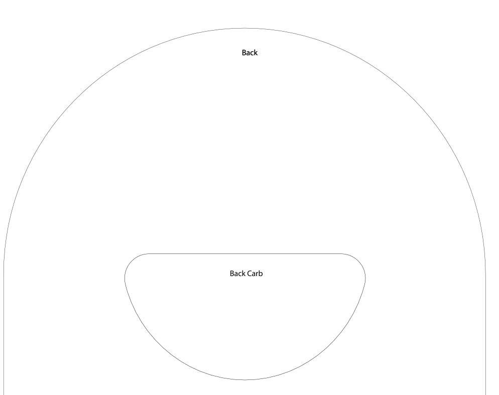
Dimensions Ford 351C Bottom Plate Back to Back Carb 4 11/16 inches Back Carb to Center Carb 4 5/16 inches Center Car to Front Carb 5 inches Back carb to Front Carb 9 5/16 inches Bottom plate 21 inches long and 10 inches wide
