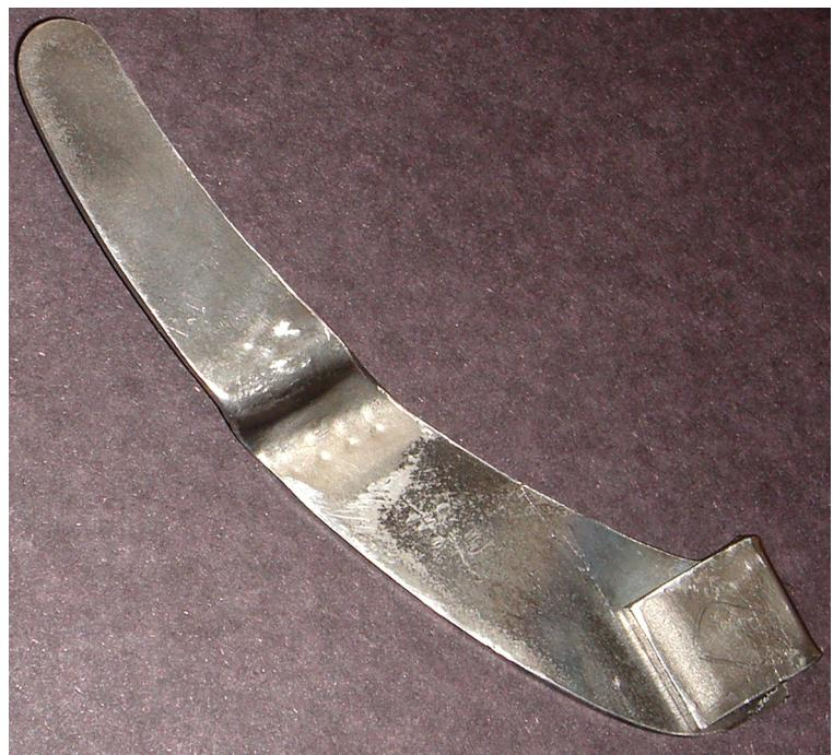
The arm was cut and shaped from 11-gauge flat steel plate. Bends were made at the end and along the arm. Not exactly up to professional standards, but should not be too difficult for a machinist to do. The template was used to mark the location of the slotted hole. Cutting the slotted hole was to be my greatest challenge, although it shouldn't have been.
