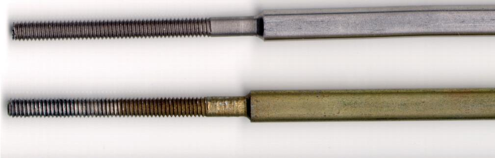
with a hacksaw and dressed the cut with a file to give it a finished look. The edges were then beveled to eliminate the sharpness.
