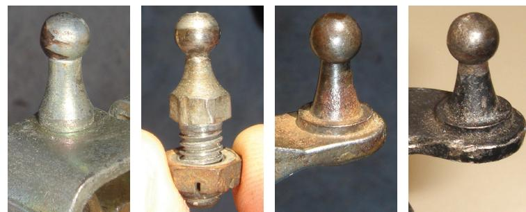
Possible ball sources, from left to right: 65 and later Galaxie carburetor throttle shaft or other cable-operated carburetors, threaded stud available in aftermarket, 64-65 Falcon/Comet link between the gas pedal rod and vertical link connecting to the accelerator bellcrank assembly, and 64-65 Falcon/Comet accelerator bellcrank assembly (the one used in this project).
