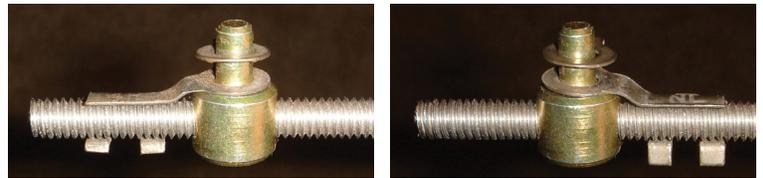
The R.H. clip attached forward on the rod (left), while the L.H. clip can also be used if attached aft. The open part of the clip must face upward to mate with the tri-power crossunder linkage.
