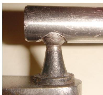
This is about the right depth for the ball to engage the socket.
