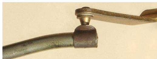
The arm and rod are connected by a ball and clip. The ball diameter measured .259" and the socket .261". The spring steel clip prevented the ball from disengaging from the socket under normal operations. The ball was secured to the arm by swaging.
