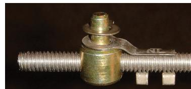
The R.H. clip attached forward on the rod (left), while the L.H. clip can also be used if attached aft. The open part of the clip must face upward to mate with the tri-power crossunder linkage.
