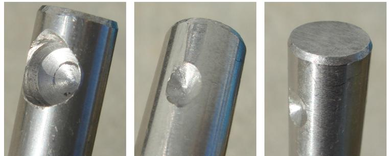
The socket hole must be sized according to the ball diameter. A dimple on the opposite indexes the clip (right). A file was used to get a flat end and beveled edge.
