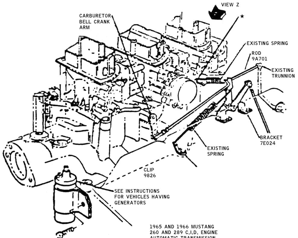
1965 AND 1966 MUSTANG 260 AND 289 C.I.D. ENGINE AUTOMATIC TRANSMISSION LINKAGE KIT NO. C4RA-9B843-E USED WITH HIGH PERFORMANCE
