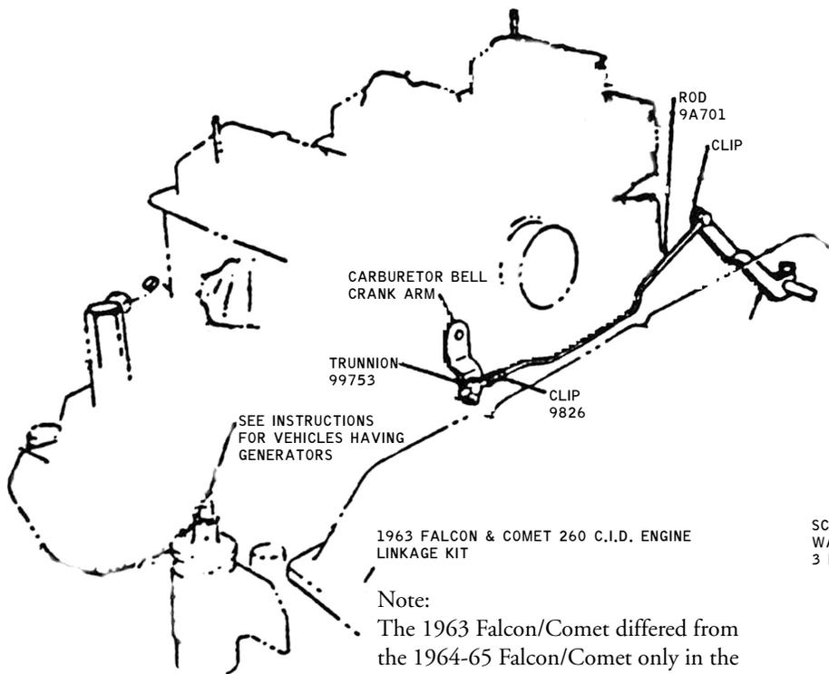
1963 FALCON & COMET 260 C.I.D. ENGINE LINKAGE KIT
