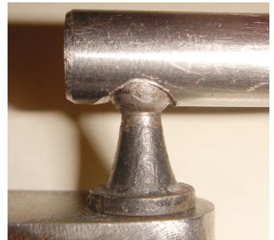
This is about the right depth for the ball to engage the socket.
