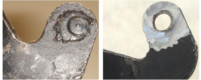
Attachment of the ball on the 65 Comet bellcrank shown above left. The dimple does not mark the center of the post. It appeared to be the impression left by the welding or brazing operation. The true center is more toward the left (centered on the extension). The weld material around the ball post was ground down, then the ball was driven free.
