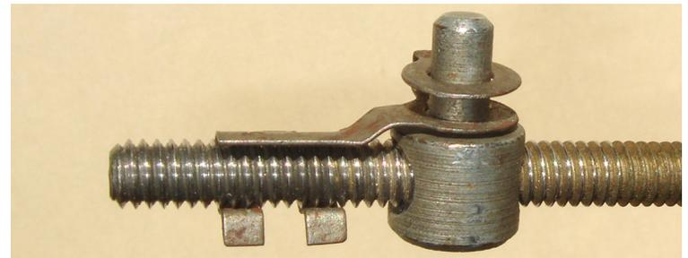
A trunnion in conjunction with a standard link clip is used to fine-tune the length of the rod.
