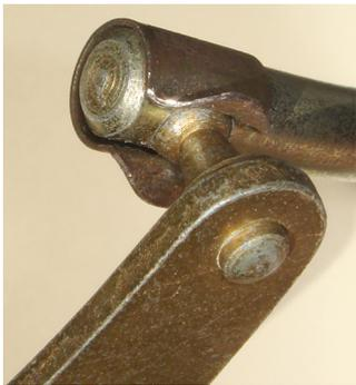
The arm and rod are connected by a ball and clip. The ball diameter measured .259" and the socket .261". The spring steel clip prevented the ball from disengaging from the socket under
