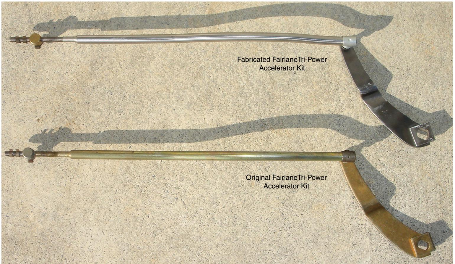
Fabricated Fairlane Tri-Power Accelerator Kit
