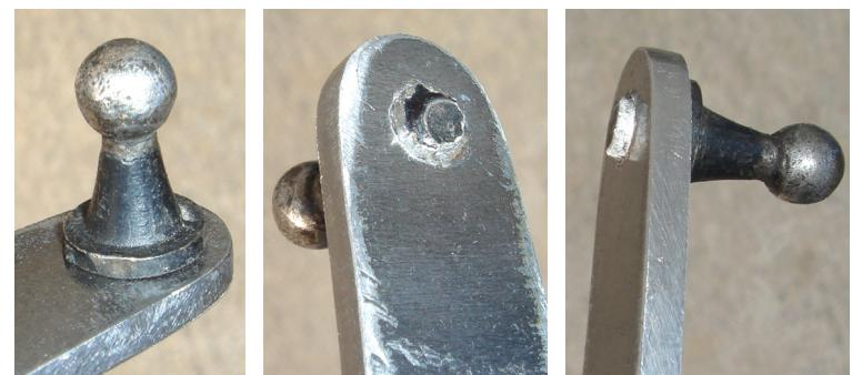
The 65 Comet ball has been pressed into the slightly tapered hole for a forced fit. The bottom of the post protruded from the back of the arm by about a sixteenth of an inch. The post could be swaged to spread the metal more tightly into the hole, or it could be brazed to the arm. In this case, brazing would give a better appearance.
