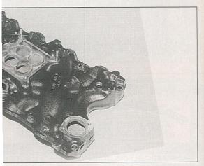
to, the stock intake manifold, all 50 lbs, 10 oz of it, generated 520.2 4 horsepower at 5000 rpm with a medium-sized hydraulic camshaft, FPA-legal truck headers. Impressive numbers considering the size and low-rise stocker or the Edelbrock Performer runners won't even cover thich is just as well since neither intake was engineered for high-rpm,
