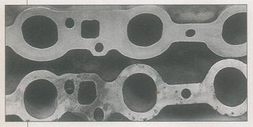
Although its spiked horsepower curve is representative, the Offy's power did not fall off sharply after the peak like a traditional single plane manifold. We suspect its comparatively smaller cross-sectional runner area helps maintain a higher air velocity which also improves low-end throttle response. In fact, the Offy's nearly straight runners (top) are actually smaller than the stock iron manifold's.
