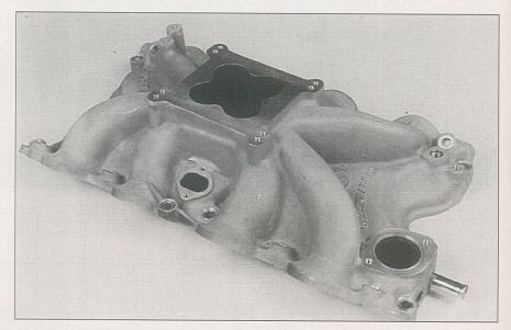
The Offenhauser 6157 single plane manifold generated more torque at the same rpm but less horsepower at a lower engine speed than the FPP4250B. The 518.4 peak torque value came at 4750 rpm. Horsepower leveled off at 507.3 at a comparatively low 5500 rpm. That's exactly opposite of what the engineering handbook says will happen, but that's why dyno testing is important. Still, both intakes are very close to each other in peak performance.
