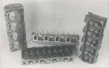
These dyno tests narrow down the performance value of race porting a pair of stock iron 429/460 cylinder heads. We first dyno tested a pair of stock iron heads, then without making any other changes, replaced them with a pair of ported heads equipped with larger valves. And, to see how the ported stockers stack up, we installed a pair of race-prepped Motorsport A429 aluminum CJ heads on the 460 dyno mule, again without making any other changes.
