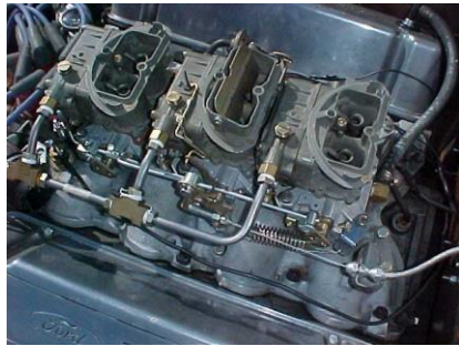
Figure 2 Author's 429SCJ 6V Carburetion with Holley List 4782/83 Carburetors
