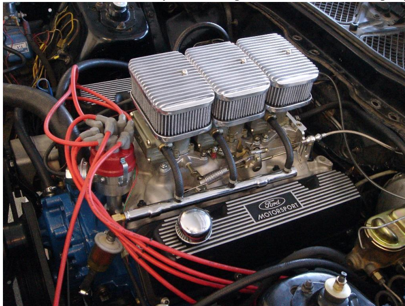
Figure 1 Ford 351C 6V Carburetion with O'Brien Trucker's Air Cleaners
