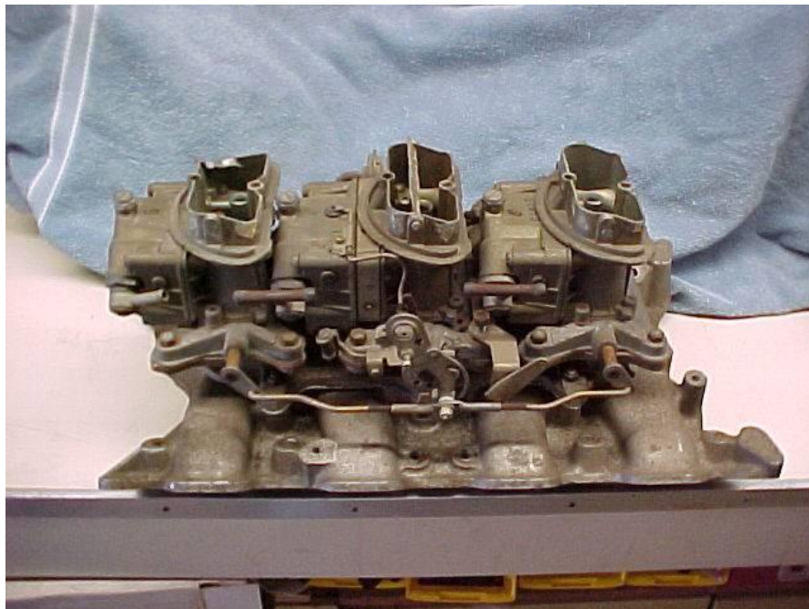
Figure 4 351C Interchangeable Intake with 6V Top Plate and Corvette Holley 2300 Carburetors
